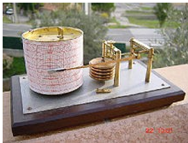
Figure 5 -Barograph using five stacked aneroid barometer cells.
