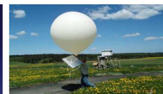
Weather Balloon (This weather balloon will rise into the atmosphere until it bursts. As it rises, it will gather weather data and send them to the surface.)
