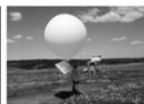
Weather Balloon (This weather balloon will rise into the atmosphere until it bursts. As it rises, it will gather weather data and send them to the surface.)
