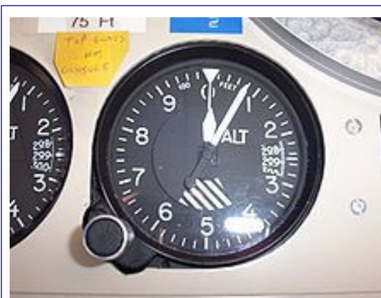
Figure 2 - Kollsman-type barometric aircraft altimeter as used in North America displaying an altitude of 80 ft (24 m).
